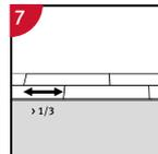
**7** Staggered joint distance i.e. minimum distance between short ends of planks in parallel rows shall not be less than the given length.
