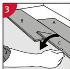
**3** Fold the panel down in a single movement. During the fold down, make sure the panels are close to each other.
