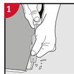
**1** Remove the vertical locking part of the strip with a chisel, put applicable glue on the strip and push the panels horizontally together. Place some spacers between last board and the wall.
