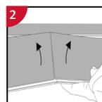
**2** Disassemble the panels by lifting the short ends upwards.
