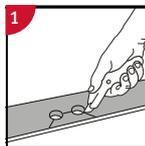
**1** Drill holes two times larger than the diameter of the pipes. Remove a piece of the panel with a utility knife. Put the panel on one side of the pipes and the removed piece on the other side.
