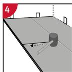
**4** Afterwards use a rubber hammer along the short end just installed.
