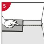
**5** At the end of the first row, put a spacer to the wall and measure the length of the last panel to fit.
