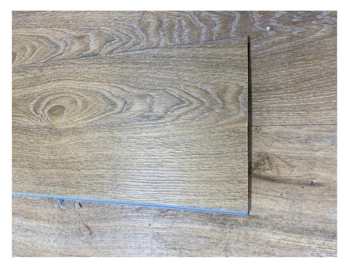
In addition to this, the original two boards fit together perfectly with the brand new board we were comparing them to. The image below shows the three boards fitted together, with the two boards used for testing to the middle and right hand side.
