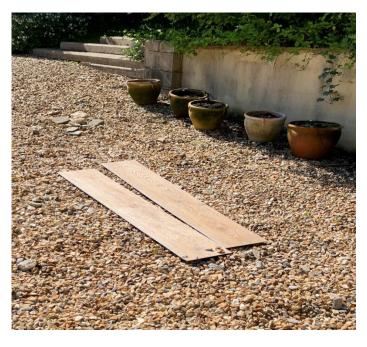
The two boards - placed on a gravel driveway last July - were left exposed to the soaring temperatures of Summer 2019 which then quickly changed to a wet and harsh winter, with the boards at some points even being covered in snow.
